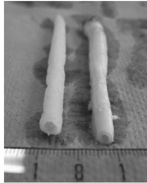
Figure 3-4: Photograph of a porous tubular PTMC structure (left, sample A-50) and a porcine carotid artery (right).
